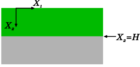
Fig.S1. Consider a piece of elastomer compressed under generalized plane strain condition. The hydrogel has a free surface on one side and is bounded at the other side. Set up a Cartesian reference system with X_1 along the surface of the hydrogel and X_2 pointing from the free surface towards the bounded surface. The bounded surface locates at X_2 = H , where H is the thickness of the hydrogel in the reference configuration.
