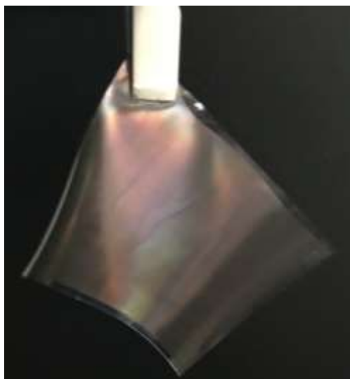
Figure S6. Optical image of a pre-strained 7-nm-thick Au film ( \lambda_{pre}=1.5 ). The substrate is PDMS. The scale is about 3 cm \times 5 cm.
