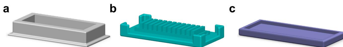
Figure S6. 3D-printed mold for casting the pneumatic soft actuator. a) Outer mold of multi-chambered upper section b) Inner mold of multi-chambered upper section c) Mold for strain-limiting base layer.
